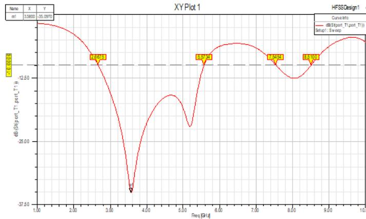
**Figure 7.** Simulated  $S_{11}$  parameter of kite shaped array configuration.
