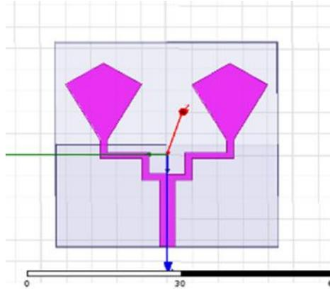
**Figure 4.** Simulated kite shape array for patch design
