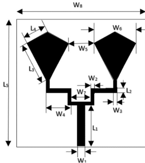
**Figure 2.** Kite shaped array for patch design.
