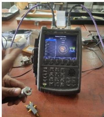
**Figure 6.** Experimental setup using VNA (Agilent Technologies, FieldFox, Model No. N9925A up to 9GHz) for optimized antenna.
