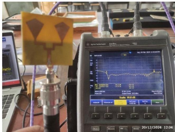
**Figure 8.** Experimentally measured  $S_{11}$  parameter through VNA
