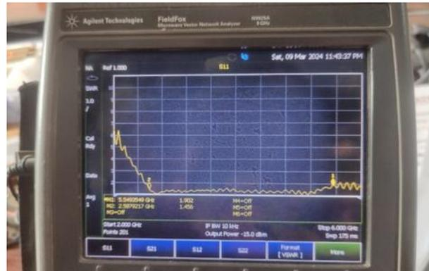
Figure 10. Measured VSWR of fabricated array antenna.
